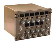
The 5701 series of Audio Control Panel is standard equipment aboard the 777 and 767-400 aircraft. The panel features a full liquid seal which eliminates the harmful effects of coffee spills. The panel communicates to AvtechTyee's 5700 series of Audio Management Unit via an ARINC 429 data bus. All lighting is accomplished via LEDs.
