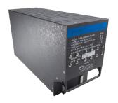
The 5700 series Audio Management Unit (AMU) is standard equipment aboard the Boeing 777 and 767-400 aircraft. The system is fully digital whereby the Audio Control Panel communications to the AMU are based on the ARINC 429 communications protocol and the audio is handled in the digital domain within the AMU. The system features a full wraparound BITE audio injection test with BITE reporting via the ARINC 629 bus or discrete outputs.
