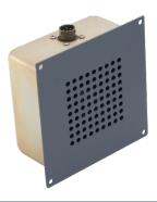
The 5064 series of speakers are 8 ohm, 9 Watt five inch speakers housed in an aluminum enclosure with an integrated connector. The 5064 speaker is used by Bombardier for the deHaviland Dash 8 aircraft and the RJ series of regional jets.
